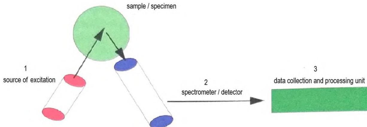
Fig. 4. EDXRF analyzer subsystem
