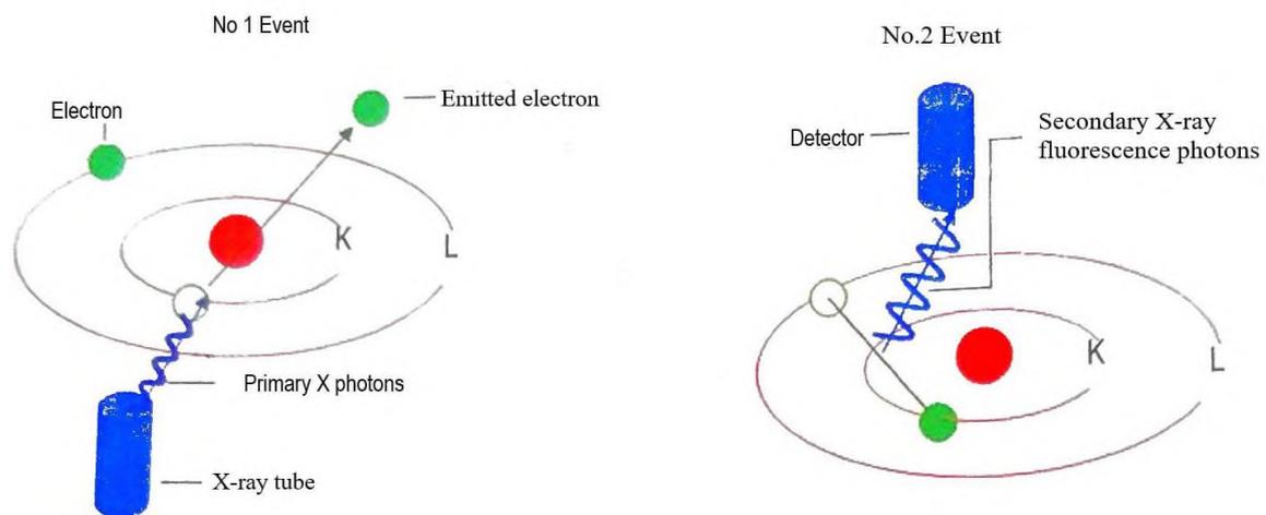
Fig. 2 The principle of fluorescence
