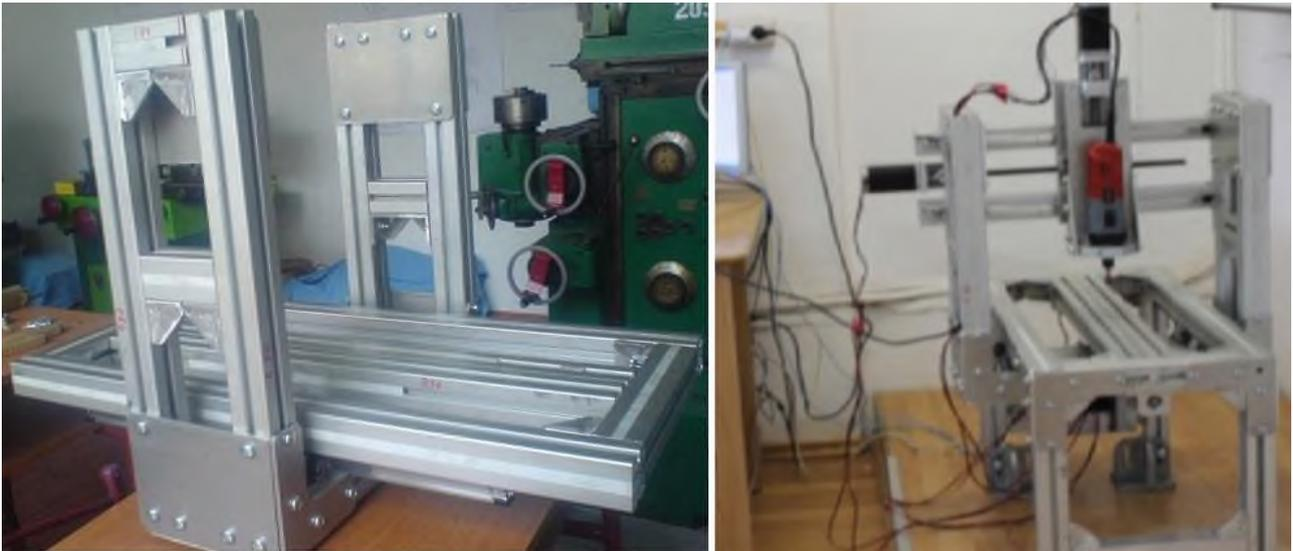
Figure 8. The way in which the milling machine with numerical control along three axes is implemented
