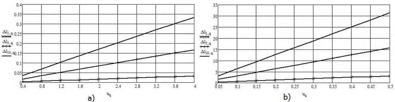
Figure 6. Influence of axial and radial wear of the drum grooves on the cable elongation
