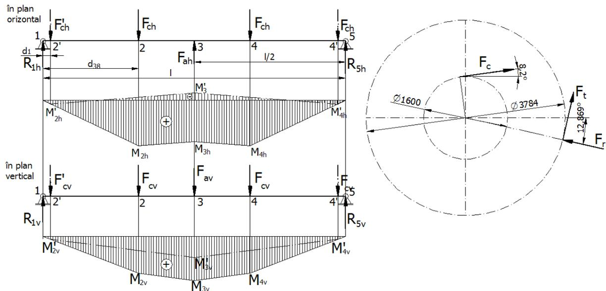
Figure 4. Calculation model of the cable winding drum
