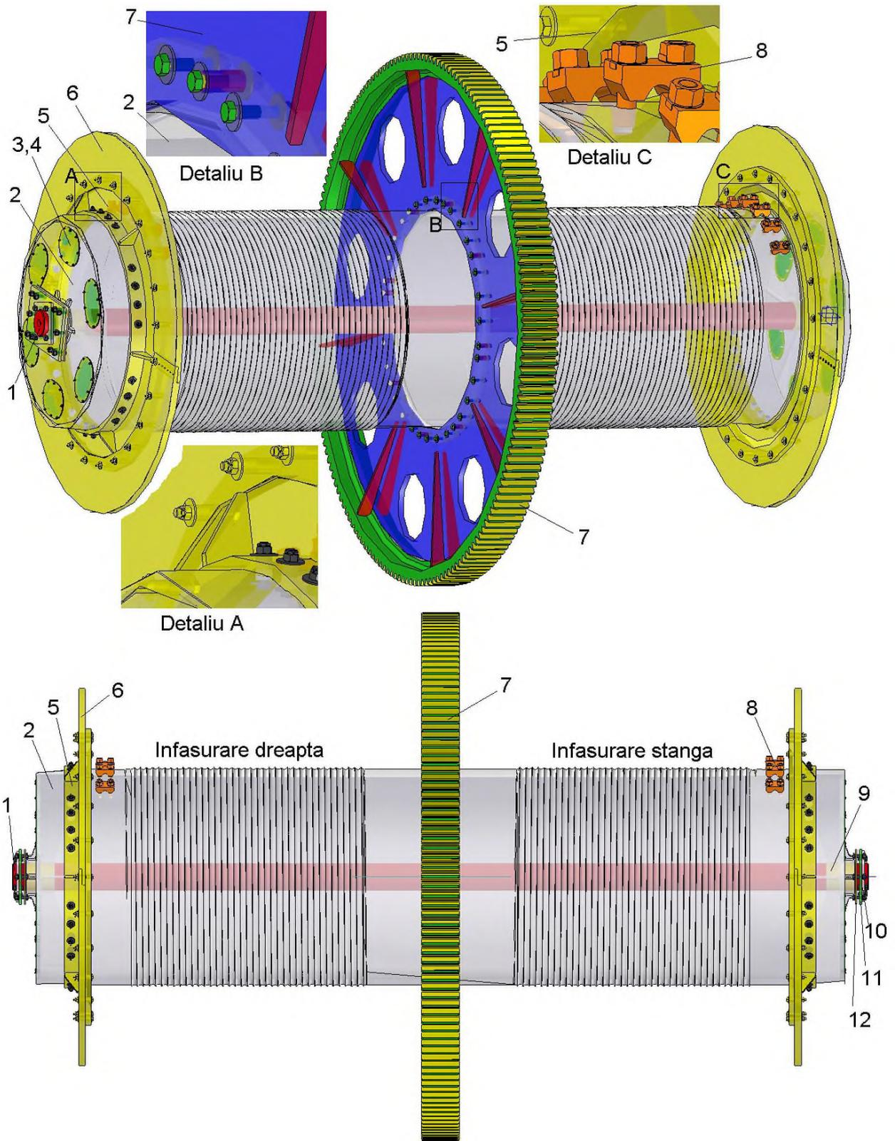
Figure 8. Overall solution for the drum with brake disks – variant II
