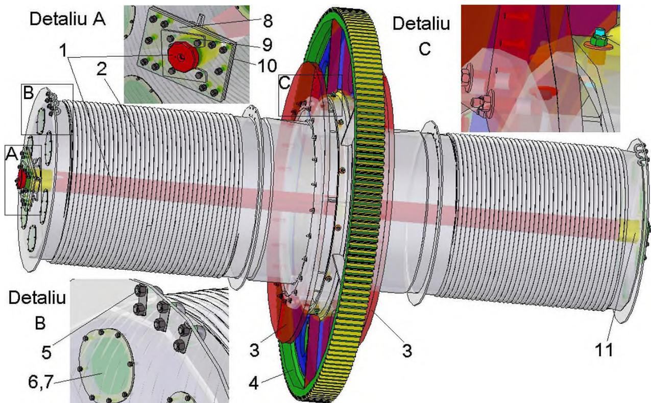
Figure 7. Overall solution for the drum for cable winding – variant I
