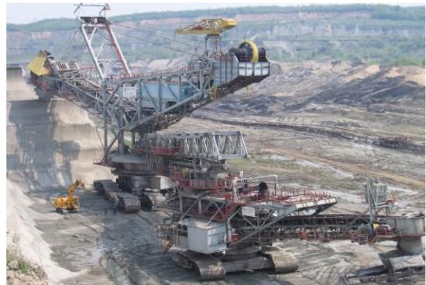
Figure 1. Overall view of EsRc-1400 bucket wheel excavator
