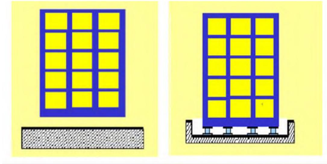
Fig.1 "The Design/consolidation method by isolating the base "
