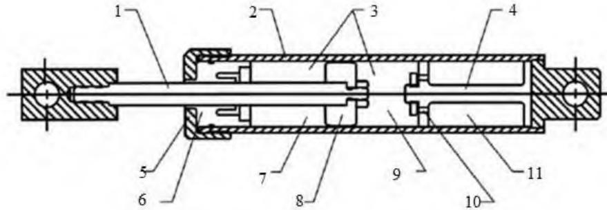
Fig. 2 The structure of a hydraulic damper with viscous liquid
