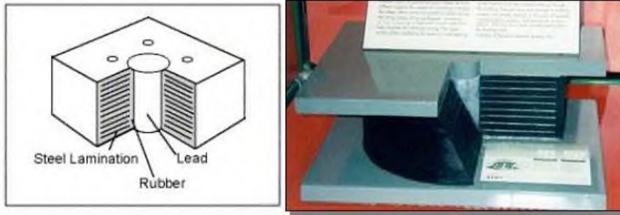
Fig 4. Rubber bearing with lead core
