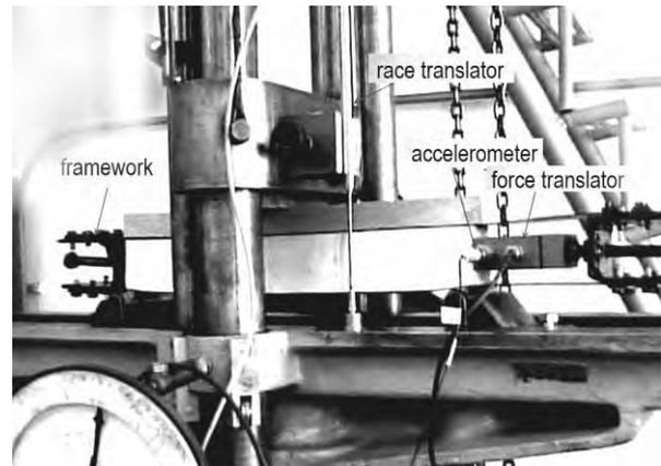
Fig. 1 Device for testing the wood beams
