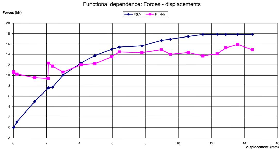
Fig.3. Beam with reinforcement and tensioning force  $F_t = 10\text{kN}$
