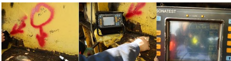
Figure 3. Wear of the screws in the joint area of section II with section III.
