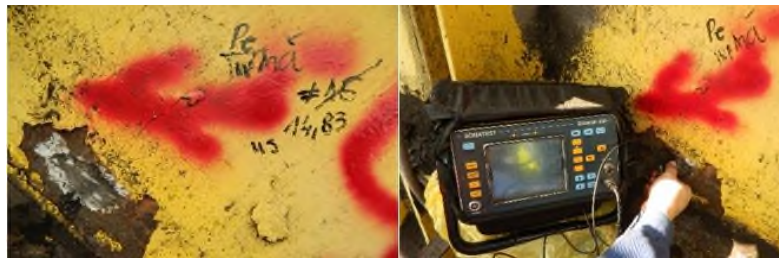
Figure 3. Material thickness control at the joint core between the platform and the balancing arm.
