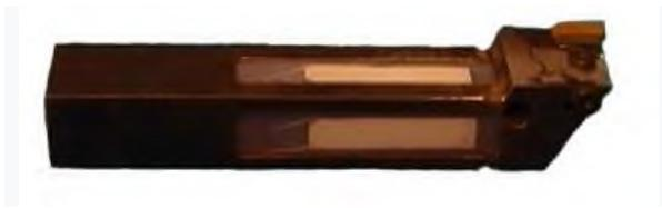
**Figure 3. The first attempt at an active tool holder solution using the piezo-ceramic technique [7].**
