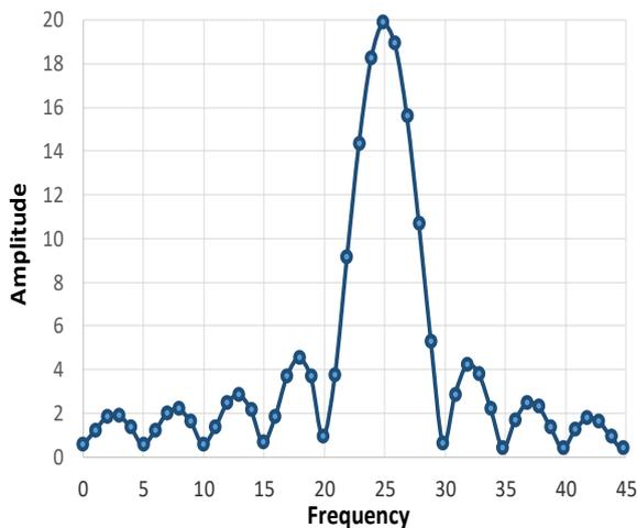
Figure 3. The spectrum for the signal segment that has just  $f_1=25.17$  Hz
