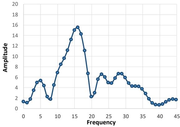
Figure 6. The spectrum for the signal segment that has portions with frequencies  $f_1=25.17$  Hz and  $f_2=15.17$  Hz as well
