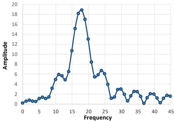
Figure 7. The spectrum for the signal segment that has portions with frequencies  $f_2=15.17$  Hz and  $f_3=19.33$  Hz as well
