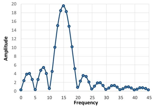
Figure 4. The spectrum for the signal segment that has just  $f_2=15.17$  Hz
