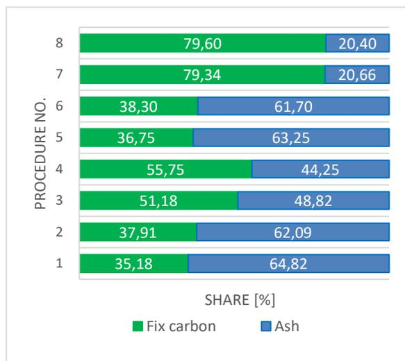
Figure 2. FCC value in CCGP following high temperature carbonization
