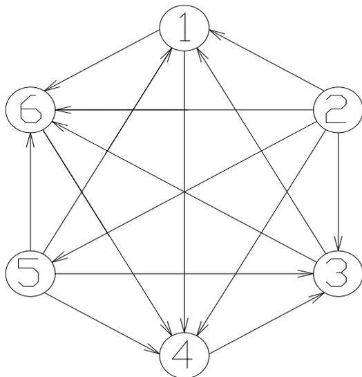
Figure 1. Example of scheduling maintenance operations by means of an oriented graph
