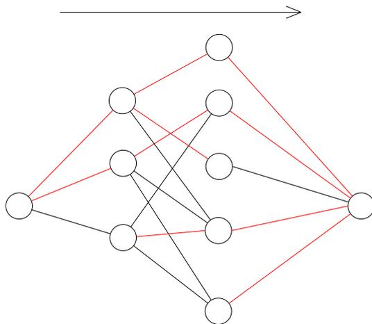
Figure 4. The matching of a bipartite graph – example with 3 operations and 5 possible operators
