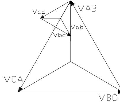
Figure 10. Phasor diagram for connection A – a (HV star point not available)
