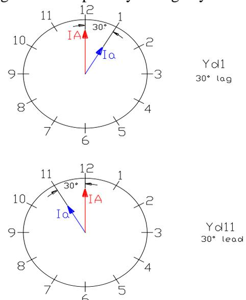
Figure 1. Phase shift for clock numbers 1 and 11 respectively for star-delta connection
