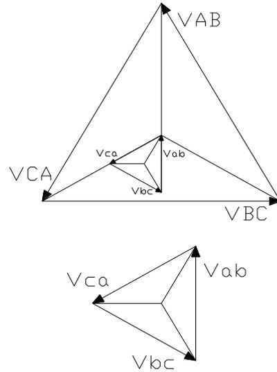
Figure 7. Phasor diagram resulting from connecting HV star point with LV phase A
