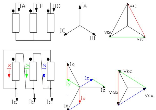
Figure 4. Yd7 vector group derived from Yd11 by swapping the LV windings polarity
