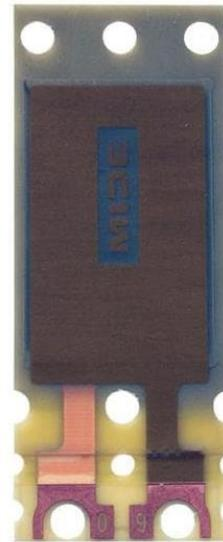
Fig.3 Piezoelectric slide
