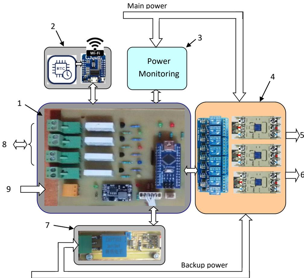
Fig.2 System structure
