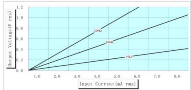
Fig.4 ZMPT101 sensor voltage characteristic
