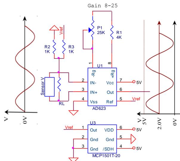
Fig.5. Circuit and signals for voltage measure
