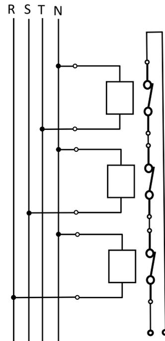
Fig.3 Lack of a phase detection circuit
