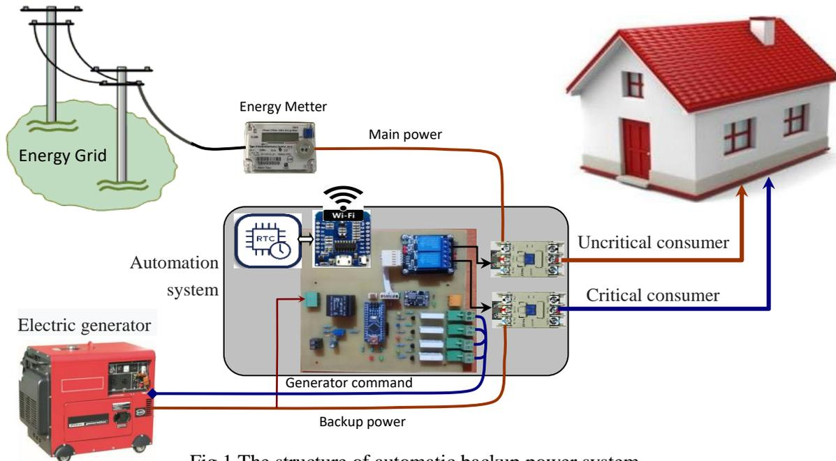
Fig.1 The structure of automatic backup power system
