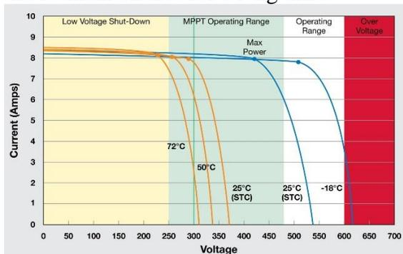
Fig.9 The influence of the temperature on the cell
