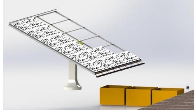
Fig.10 Active cooling system of the photovoltaic panel
