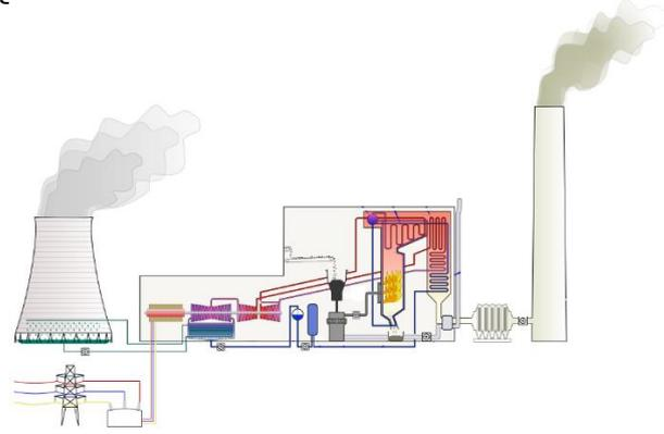
Fig.2 Schematic of thermal power plants
