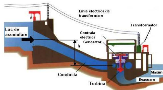
Fig.3 Schematic of hydropower plants
