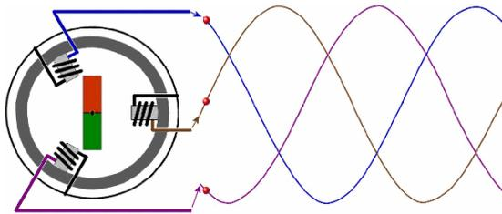
Fig.1 Principle of electricity generation
