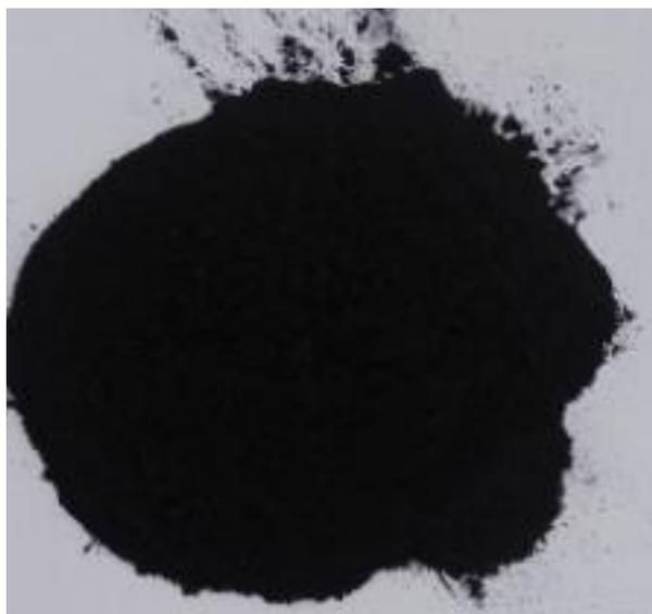
Figure 7. Highly concentrated fraction (61.38% fixed carbon content)
