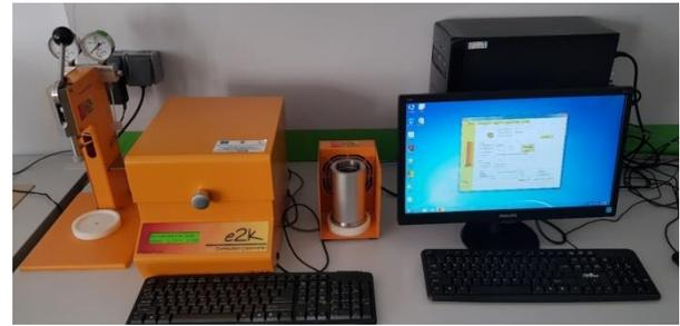
Figure 2. E2K Oxygen Bomb Calorimetric System
