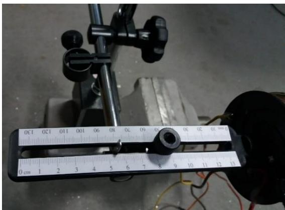
Figure 2. Coil fixed on adjustable mounting bracket
