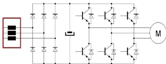
Figure 1. AC line reactor applied
