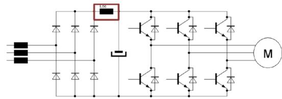
Figure 3. DC link coil applied
