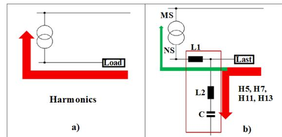
Figure 5. Passive harmonic filter a.) not applied b.) applied
