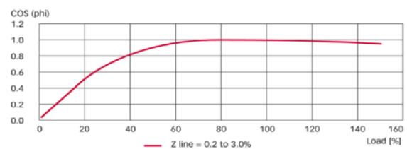
Figure 6. Performance curve passive harmonic filter
