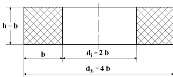
Figure 2. Optimum coil dimensions without ferromagnetic core
