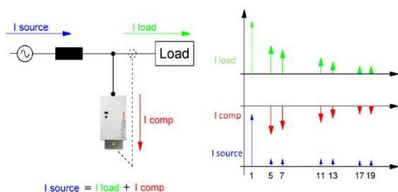
Figure 7. Function of an active harmonic filter
