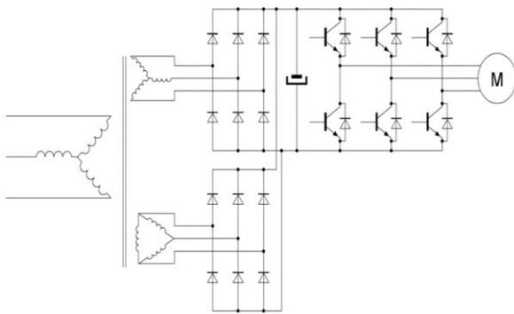
Figure 4.12-pulse setup
