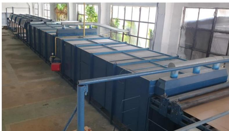
Figure 5. Belt conveyor for PVC baking
