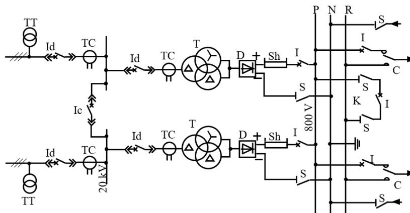
Figure 5. Schematic diagram of a substation to supply the urban traction system.
