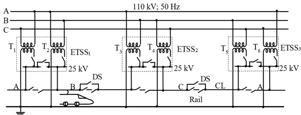
Figure 1. Electricity supply scheme for a railway section
