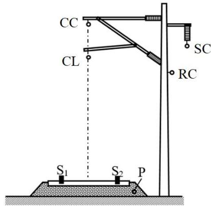
Figure 4. Circuit configuration in a  $2 \times 25$  kV electrical traction system.
