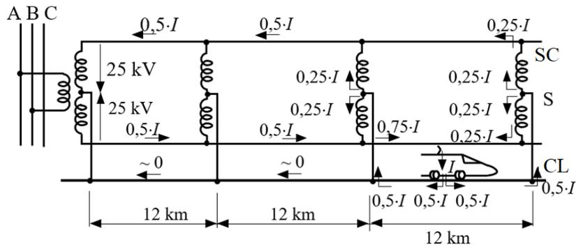
Figure 3. Typical electric current flow for  $2 \times 25$  kV system.
