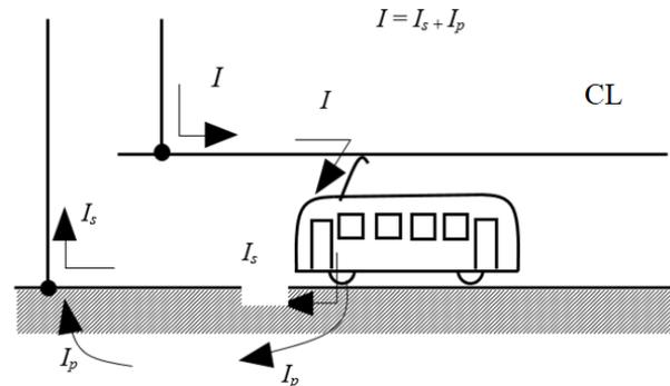
Figure 6. Circulation of electric current absorbed by urban rail vehicle.
