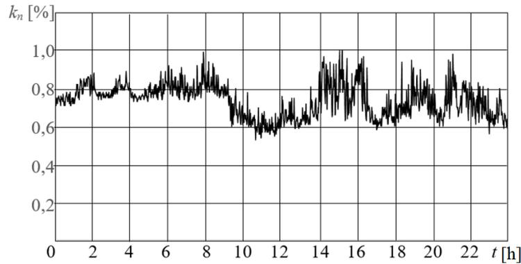
Figure 2. Variation of the negative non-symmetry factor  $k_n$  during one day at 110 kV busbars feeding an electric traction substation ( $k_{n50\%} = 0,75$ ;  $k_{n95\%} = 0,88$ ;  $k_{n5\%} = 0,63$ ;  $\sigma = 12\%$  ).
