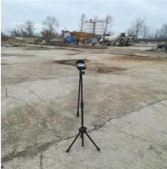
Fig. 5. Location of the Bruel & Kjae 2250L sound level meter used to monitor the noise level
