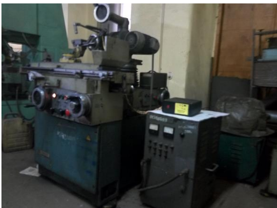
Fig. 2. EDDFG set up assembled on EDM machine
