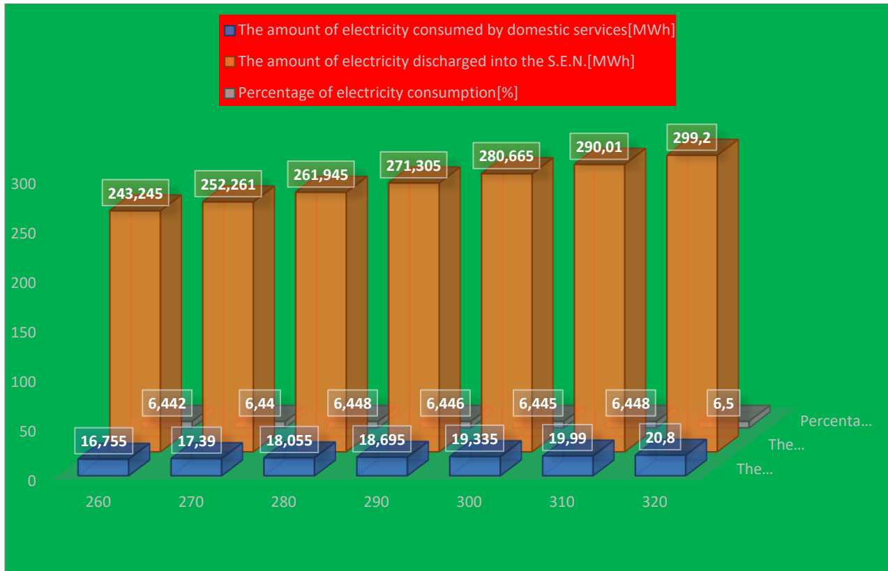
Figure 1. Dependence between the amount of electricity produced and the electricity consumption of domestic services
