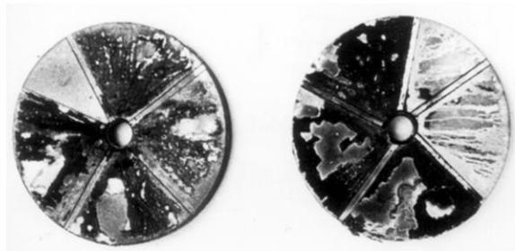
*Fig. 1 Aspect of some samples after nitriding*
