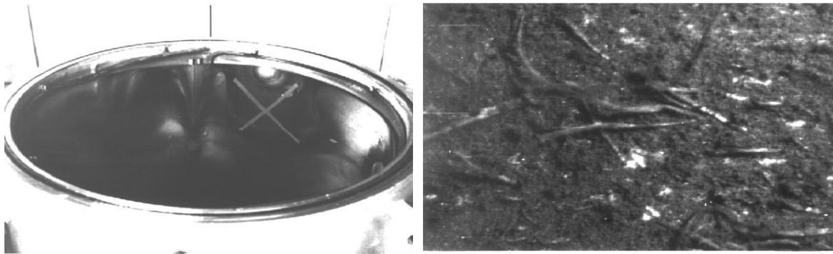
*Fig. 1 Deposits formed on the surface of the recipient's walls during nitriding*
