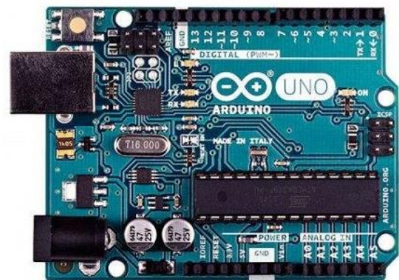
Figure 3. Arduino UNO development module [14]
