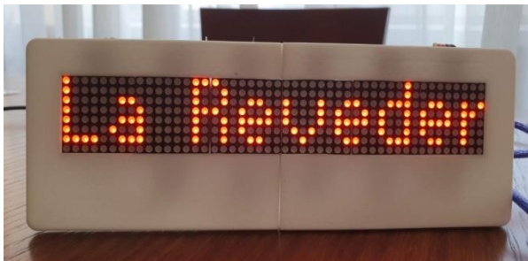
Figure 14. Testing the light advertising system for displaying the text "Goodbye"
