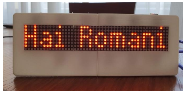
Figure 10. Testing the light advertising system for displaying the text "Hai Romania"
