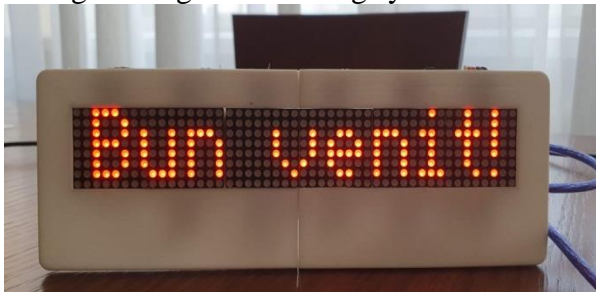
Figure 13. Testing the light advertisement system for displaying the text "Welcome!"
