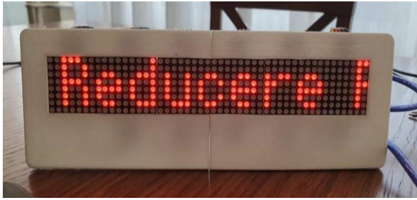
Figure 12. Testing the light advertising system for displaying the text "Discount"
