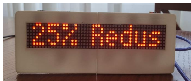
Figure 10. Testing the light advertising system for displaying the text "Hai Romania"
