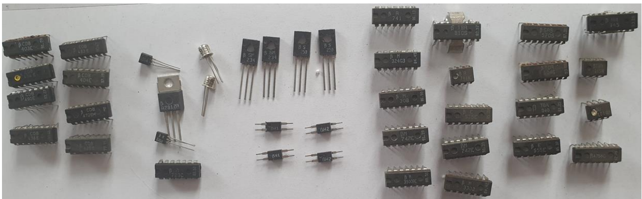
Figure 7 Logic integrated circuits from the TTL family, sensors and linear bipolar integrated circuits produced at IPRS Baneasa
