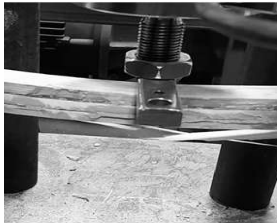
Figure 4. Failure mod of reinforced beam type I (detail)
