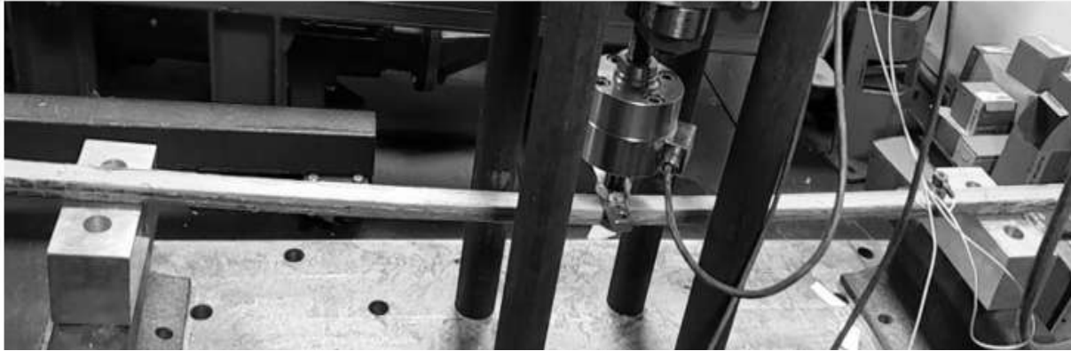
Figure 9. Reinforced beam type II – bending test
