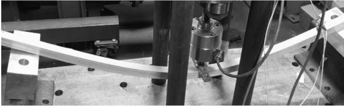
Figure 1. Unreinforced beam type I – bending test
