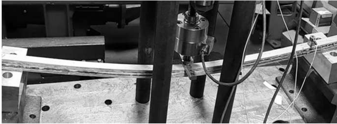
Figure 3. Reinforced beam type I – bending test
