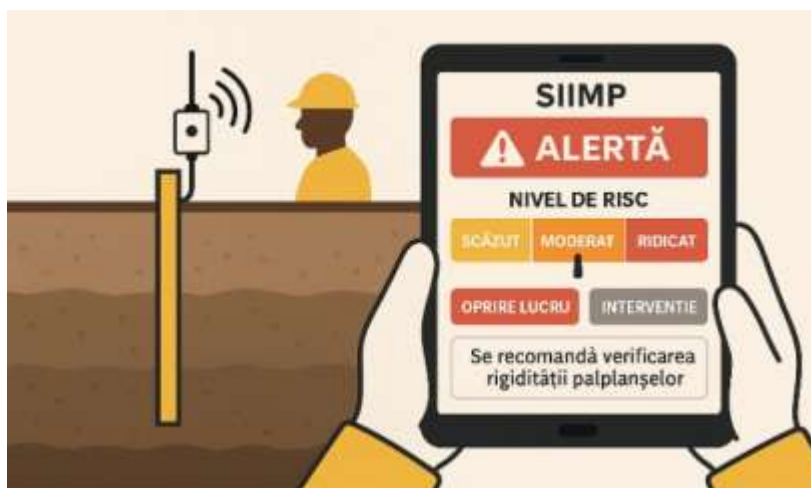
Figure 4. Occupational health and safety interface (with emphasis on alerts, colored risk levels, intervention buttons and preventive recommendations) of Intelligent Integrated Pile Monitoring System (IIPMS)
