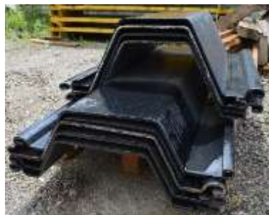
Figure 1. Examples of metal sheet piles and types of joints
