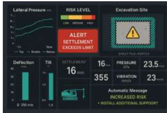
Figure 5. The technical interface of the "industrial dashboard" type (with graphs, risk bars, excavation map, numerical indicators and automatic messages) of Intelligent Integrated Pile Monitoring System (IIPMS)
