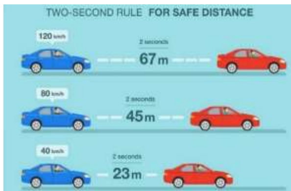
Figure 3. The safe distance between two vehicles driving in the same direction [26]
