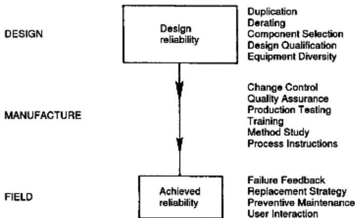
Fig.1 The complete chain of reliability
