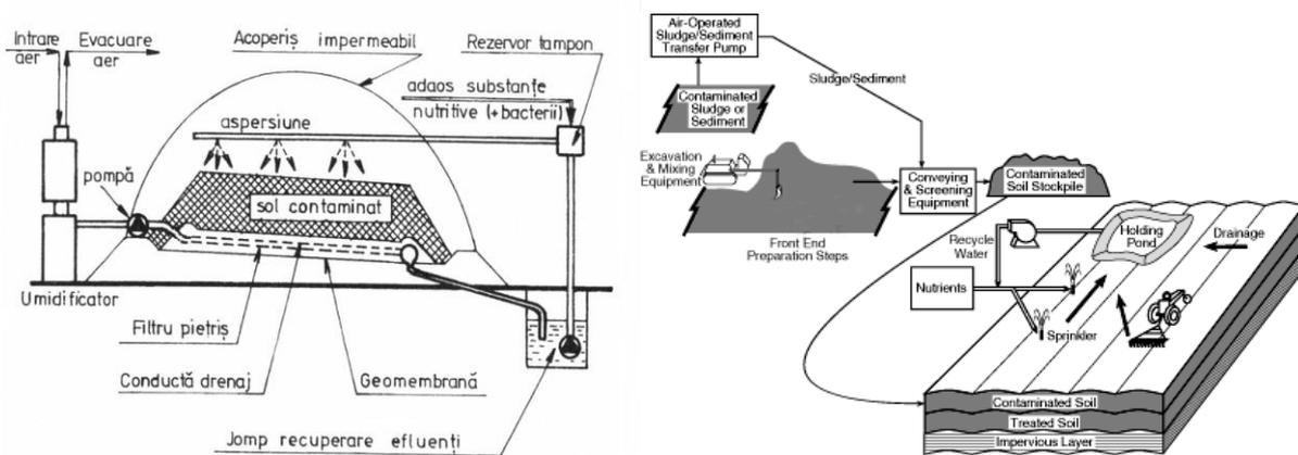
Fig. 2. Biopiles technology for bioremediation of soils polluted
