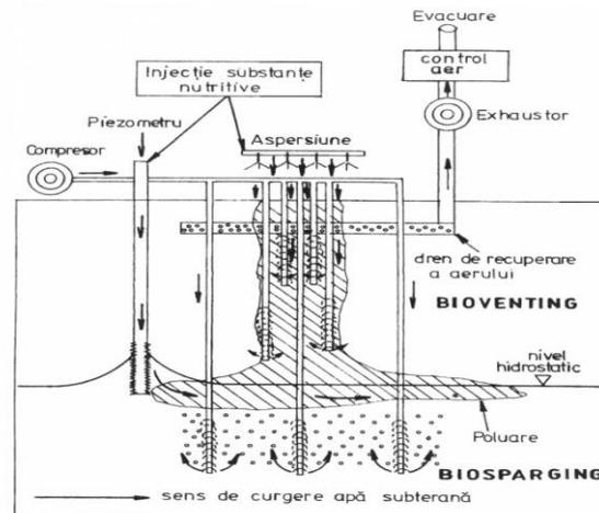
Fig. 6. Application technology biosparging site the remediation of soil
