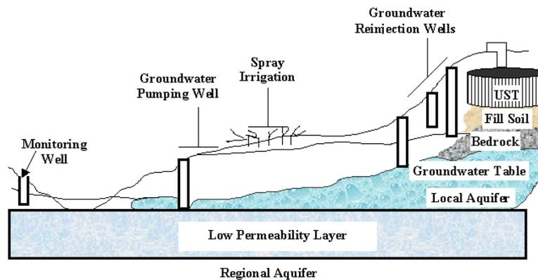
Fig. 8. Technology biostimulation and bioaugmentation polluted soil
