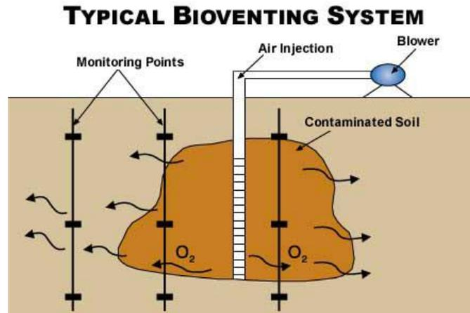
Fig. 5. Application technology bioventing site the remediation of soil
