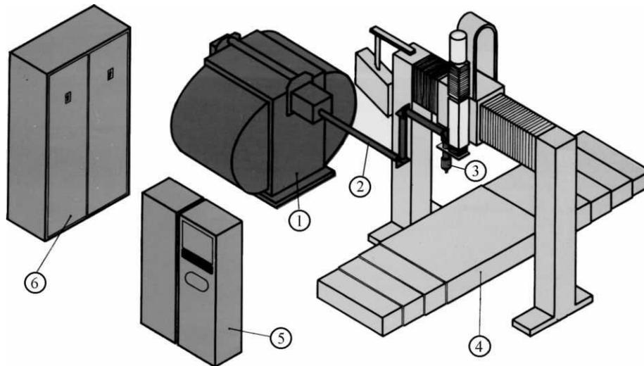
**Fig. 2:** The basic configuration of laser cutting machine:
