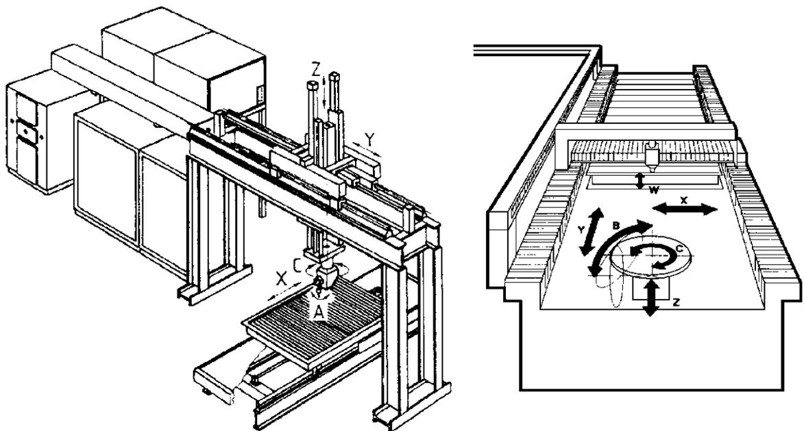
Fig. 4: Laser cutting machines for 3-D parts
