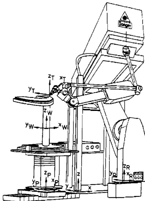
Fig. 5: Laser robot
