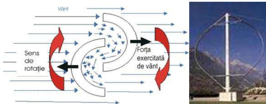
Fig. 7. Schematic diagram of Savonius rotor and image of a Darrieus wind
