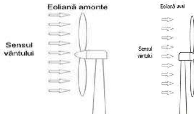
Fig. 8. Scheme horizontal axis wind turbines upstream and downstream
