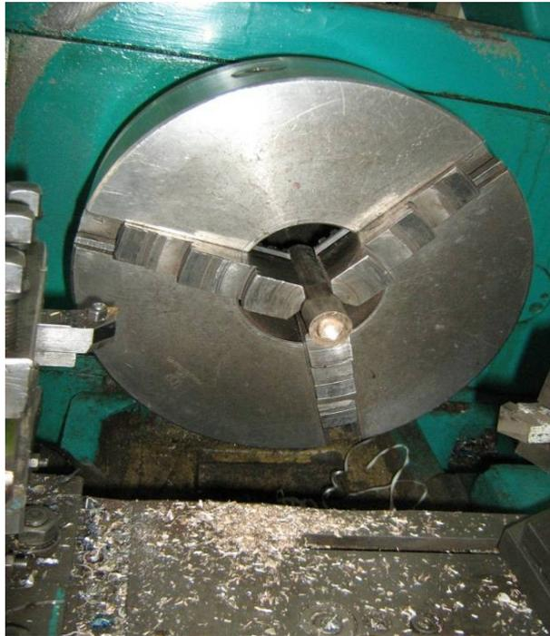
Fig. 5. A detailed view with the product fixed in the spindle head stock of the universal lathe machine
