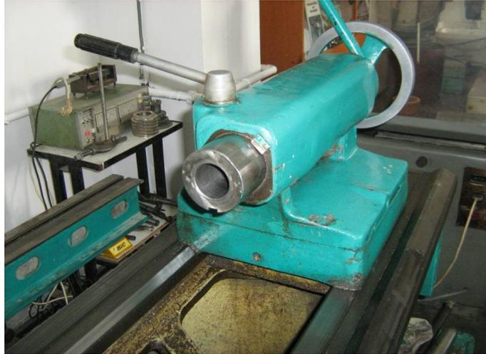
Fig. 3. The movable boring head, where the tool will be fixed
