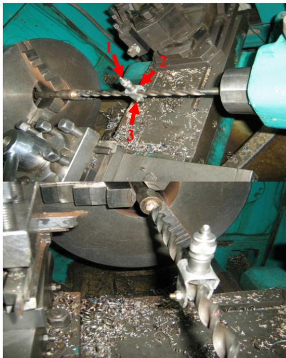
Fig. 6. A special removable assembly used to connect the accelerometer on the tool
