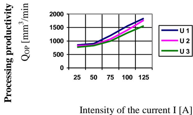
**Fig. 2:** The influence of the intensity of the I current on the  $Q_{OP}$  processing productivity for the values of the voltage  $U_1 = 28$  V;  $U_2 = 24$  V;  $U_3 = 20$  V.
