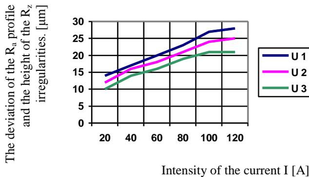
**Fig. 3:** The influence of the I current intensity on the R<sub>z</sub> irregularities height for the values of the voltage: U1 = 28 V; U2 = 24V; U3 = 20 V.
