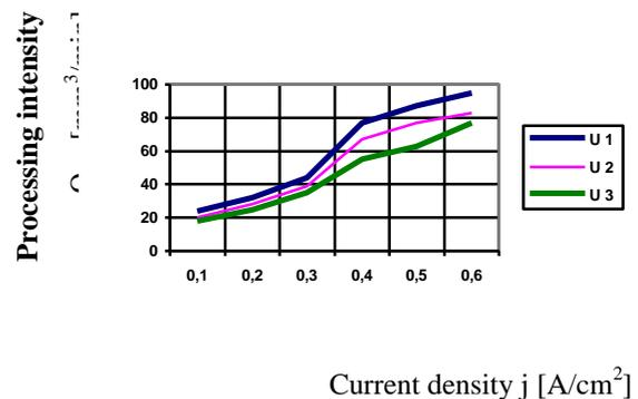
**Fig. 4:** The influence of the j current density on the productivity of the Q<sub>OP</sub> processing for the values of the voltage U1 = 28 V; U2 = 24 V; U3 = 20 V.
