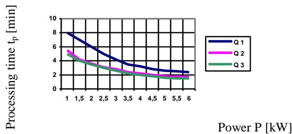
**Fig. 5:** The influence of the induced power in SL on the cutting time  $t_p$  for the values of the  $Q_1 = 30$  l/min;  $Q_2 = 25$  l/min
