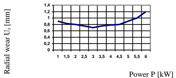
**Fig. 6:** The influence of the power induced in SL upon the radial wear  $U_r$ .
