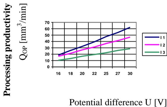
**Fig. 1:** The influence of the U difference on the  $Q_{OP}$  processing productivity, for the values of the I current  $I_1 = 40$  A;  $I_2 = 30$  A;  $I_3 = 20$  A
