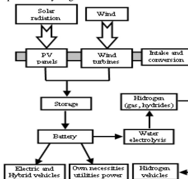
Fig. 1. Logic diagram of multiple role station which serving a 'green' highway
