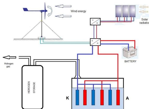
Fig. 2. The schematic diagram of hydrogen production plant using renewable energy converted in electricity
