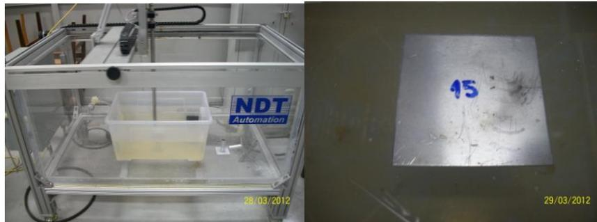
Fig.4 Ultrasonic immersion examination for the brazed pieces
