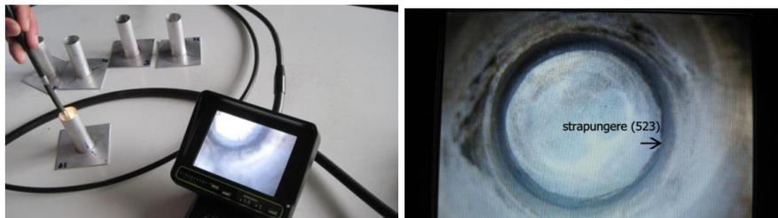
*Fig.2 Examination using the endoscope*
