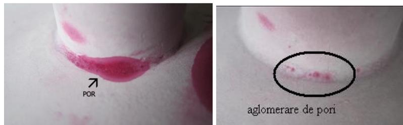
*Fig.3 Penetrating fluid examination*
