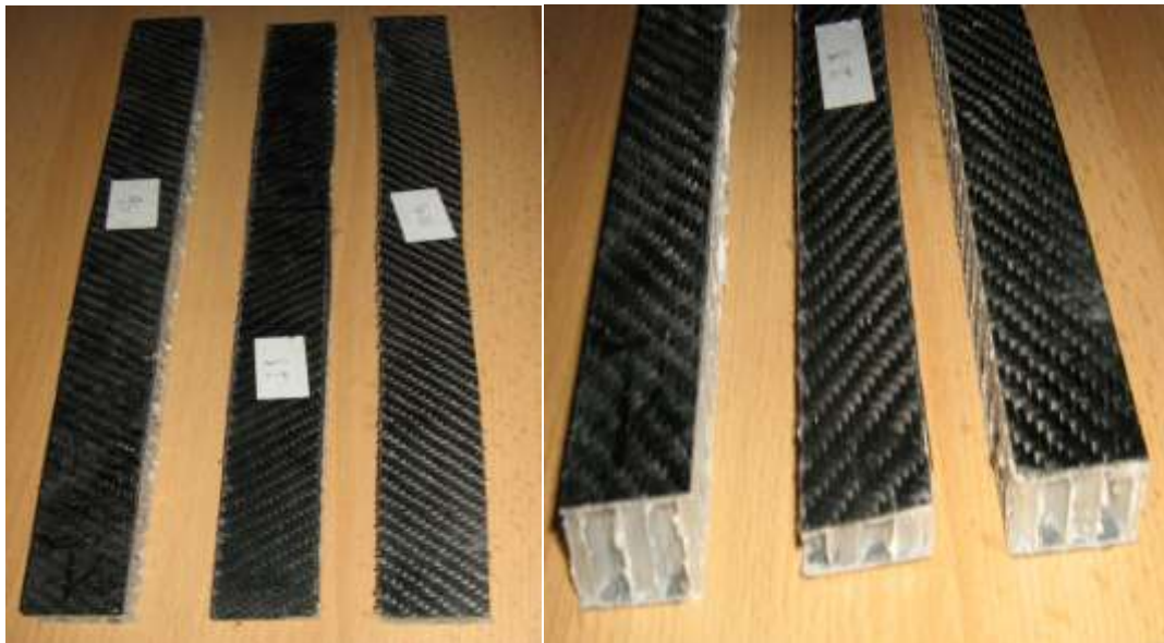
Fig. 1. Composite sandwich bars with polypropylene honeycomb core reinforced with carbon-fiber
