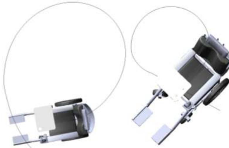
**Fig. 5.** Wheelchair motion trajectory computed in Adams.
