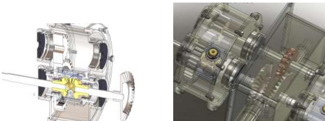
Fig. 3. Detail of a differential transmission.
