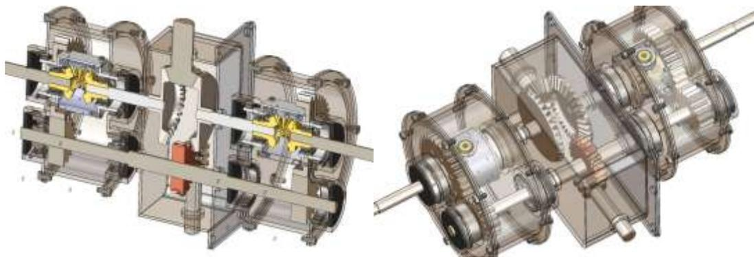
Fig. 2. Transmission assembly (with section).
