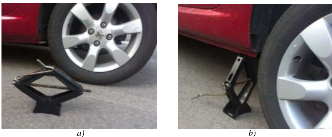
Fig. 3.1. Jack-screw with bars and gears: rest position (a) and working position (b)
