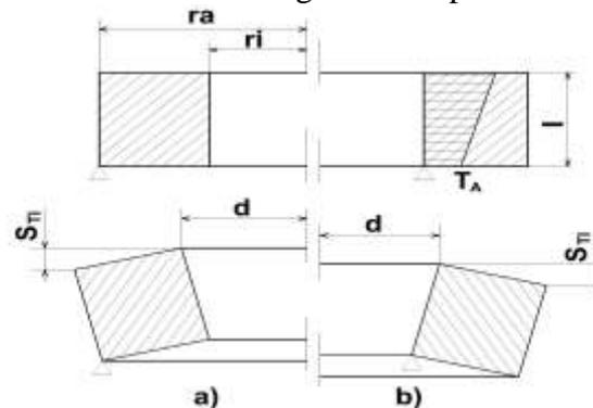
Fig.4.Deformations due to the axial temperature gradient
