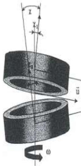
Fig.3. Primary sealing with 3 degrees of freedom
