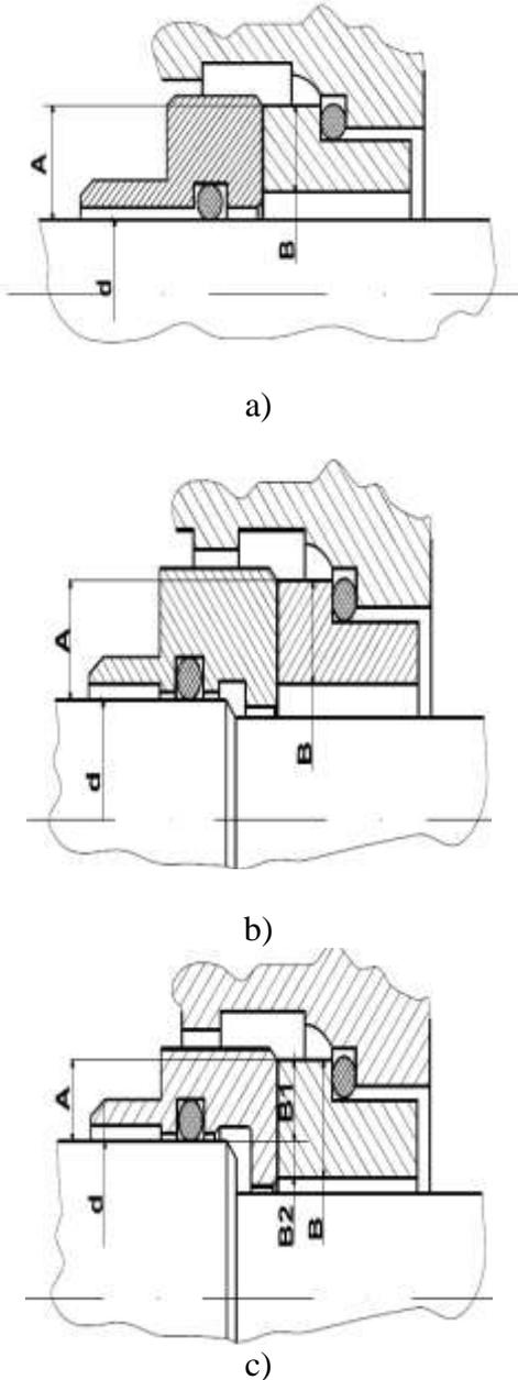
**Fig. 1.** Different arrangements of the sealing surface.
