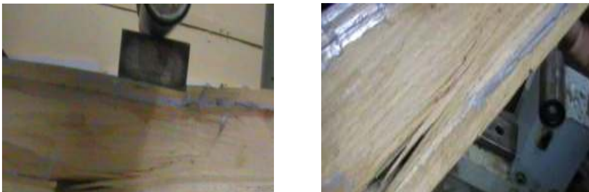
Fig. 2 Tension failure of a reinforced wood beam with two CFRP sheets and two slides of wood (up and down)
