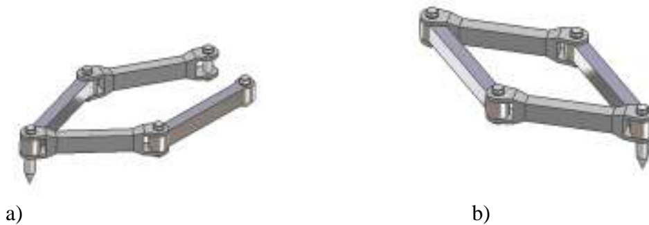
Fig. 4 Kinematic chains generators of five-bar mechanisms
