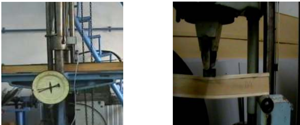
Fig.2 Universal hydraulic machine of 20 tons force, EDZ 20, with a beam reinforced with CFRP
