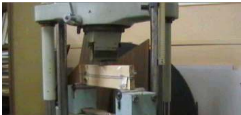
Fig. 3 Tension failure of a reinforced wood beam with two CFRP sheets (in the middle of the beam) and one slide of wood
