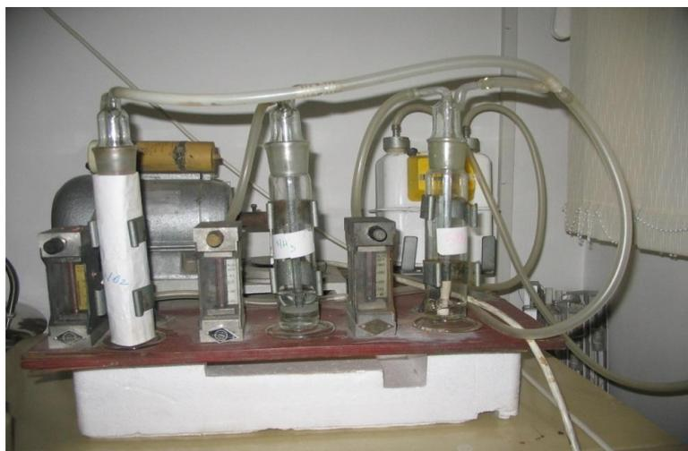
*Fig. 2 -Pump for gaseous pollutants sampling*
