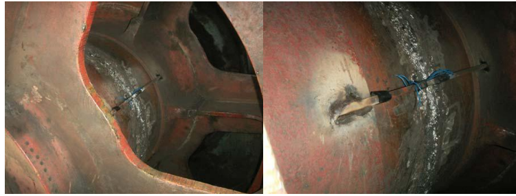
Fig. 13. Transducer welded by the two half-hubs
