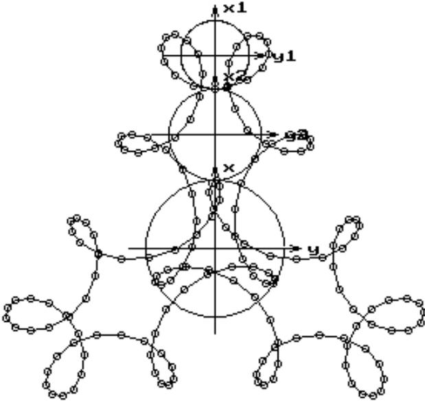
**Fig. 3.** The curve formed by rotations in a three-link gearing with the ratio  $\omega_1 : \omega_2 : \omega_3 = 4 : 3 : (-2)$  at  $\omega_1 = 3 \text{ rad/s}$
