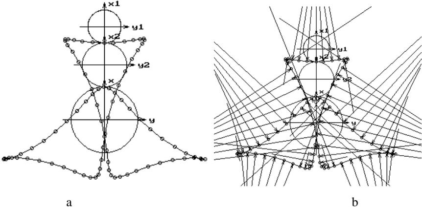
**Fig. 2.** The curve formed by rotations in a three-link gearing with the ratio  $\omega_1 : \omega_2 : \omega_3 = 4 : 3 : (-2)$  at  $\omega_1 = 1 \text{ rad/s}$  (a) and curvature vectors at its points (b)
