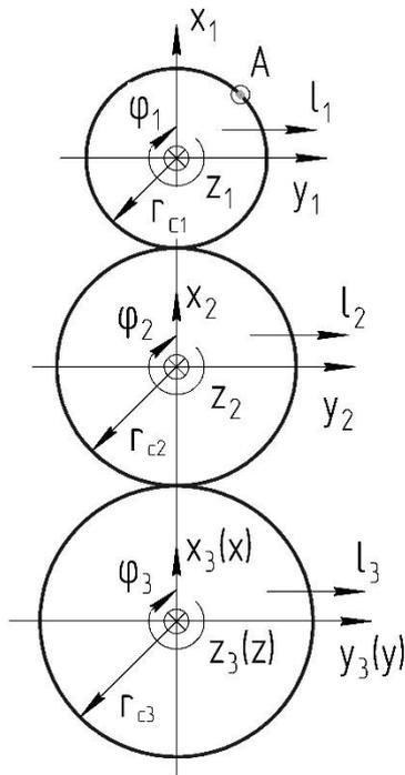
Fig. 1. The scheme of a three-members rack gearing
