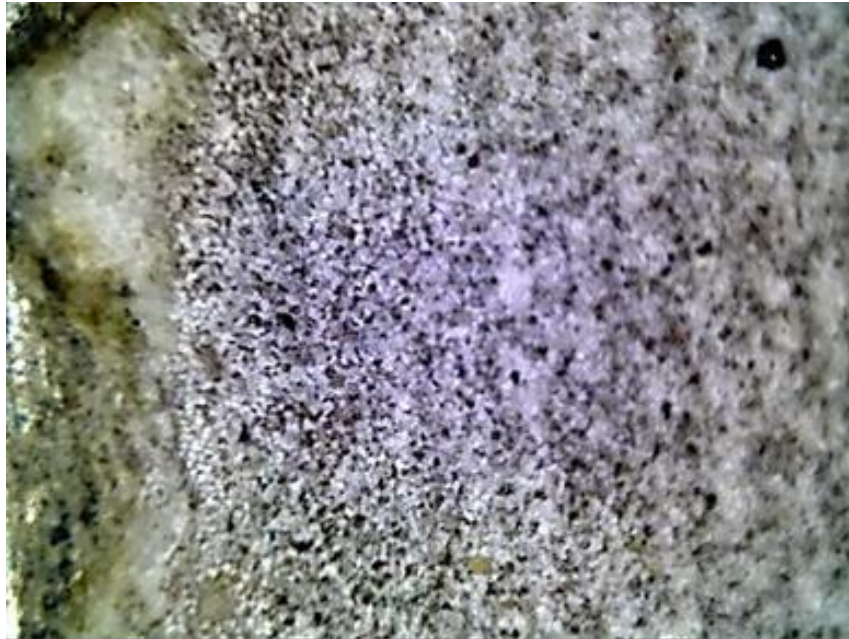
Fig. 1. Microphotographs of the framework surface of the experimental grinding wheel with a local micro-arc oxide coating on aluminum alloy AK6
