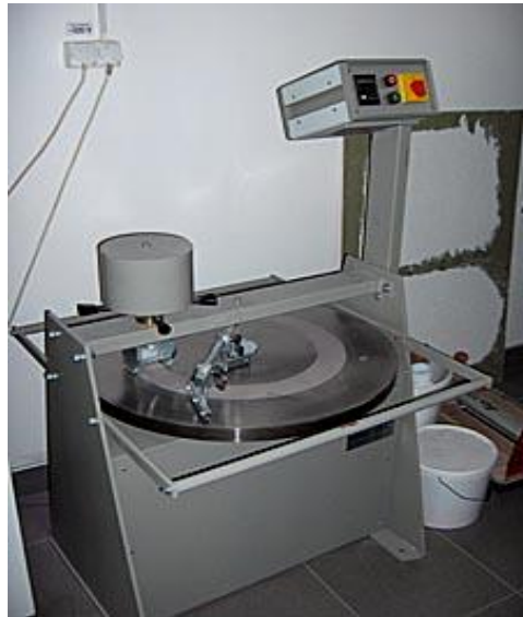
Fig.6. Stand used to determine wear resistance
