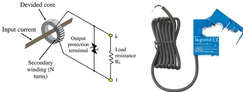
Fig.5 Clamp-type current sensor
