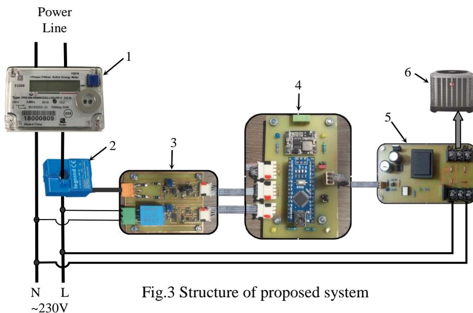
Fig.3 Structure of proposed system
