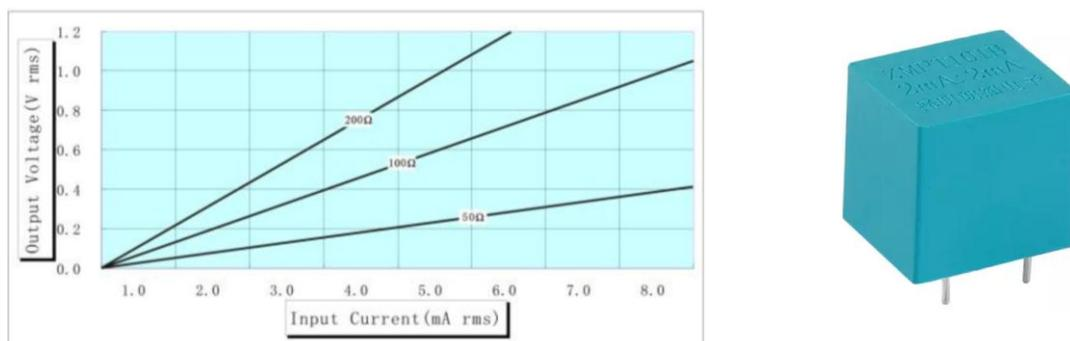
Fig.4 ZMPT101 sensor voltage characteristic
