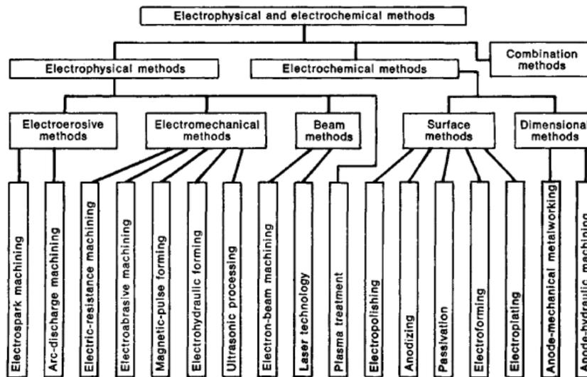
Figure 1. Classification of the principal methods of electrophysical processing
