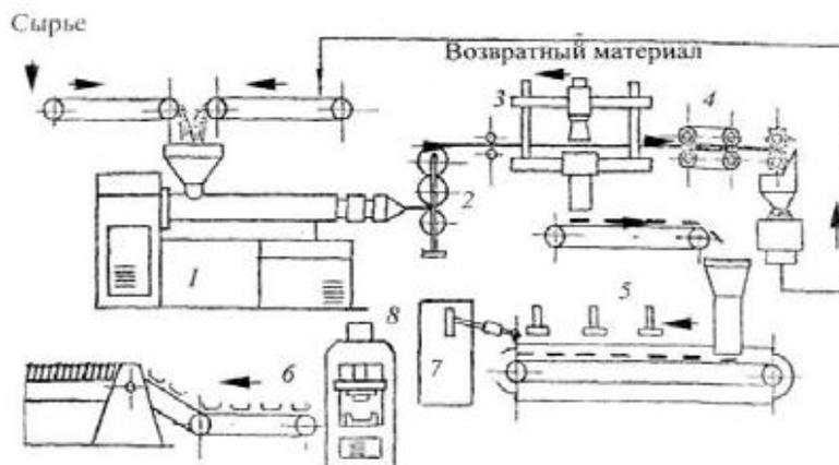
Figure 2 Scheme of obtaining products process of thermoplastics by sheet stamping, using short microwave heating: 1 - extruder, 2 - feed rolls 3 - punching device, 4 – grinder, 5 - microwave generator, 6 - transporter, 7 – manipulator, 8 - the press.
