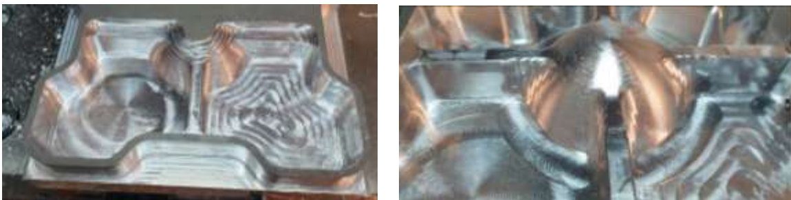
Fig 6.The part after roughing
